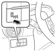
When the Blind Spot Monitoring (BSM) switch is pressed, the Blind Spot Monitoring (BSM) and Rear Cross Traffic Alert (RCTA) systems are turned off and the Blind Spot Monitoring (BSM) OFF indicator light in the instrument cluster turns on.
