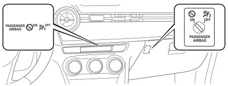
The front passenger air bag deactivation switch should be used to deactivate the front passenger front and side air bags and also the front passenger seat belt pretensioner system if installing a child-restraint system on the front passenger seat.
