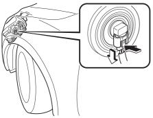
4. Turn the socket and bulb assembly to remove it. Carefully remove the bulb from its socket in the reflector by gently pulling it straight backward out of the socket.
