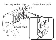
If it is at or near L, add enough coolant to the coolant reservoir to provide freezing and corrosion protection and to bring the level to F or FULL.
