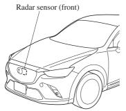
If the Smart Brake Support/Smart City Brake Support (SBS/SCBS) Warning Light (amber) is illuminated, the area around the radar sensor may be dirty. Refer to "Warning Guidance" in the centre display (Type C/D audio).
