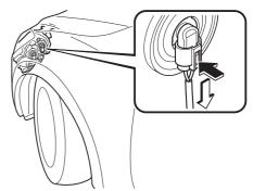
4. Turn the socket and bulb assembly to remove it. Carefully remove the bulb from its socket in the reflector by gently pulling it straight backward out of the socket.
