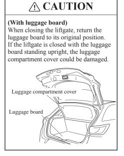
Lower the liftgate slowly using the liftgate grip recess, then push the liftgate closed using both hands.
