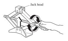
5. Place the jack under the jack-up position closest to the tyre being changed with the jack head squarely under the jack-up point.
