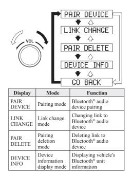
3. Press the audio control dial to determine the mode.
