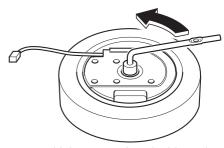
For vehicles not equipped with a subwoofer, turn the spare tyre hold-down bolt anticlockwise and remove the spare tyre.
