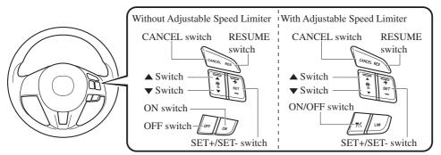
When the ON switch is pressed, the vehicle speed and the distance between vehicles while in headway control can be set. The Mazda Radar Cruise Control (MRCC) indication is shown in the display of the instrument cluster.
