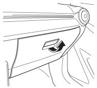
To close the glove compartment, firmly press in the centre of the glove compartment lid.
