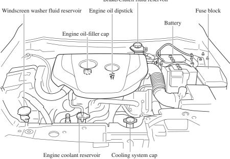
Brake/Clutch fluid reservoir
