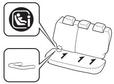
An i-Size child-restraint system can be installed to the specified seat as follows:
