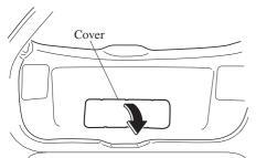
3. Using a flathead screwdriver, open the inner cover.
