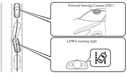
The warning light illuminates when the system has a malfunction. Refer to Warning Lights on page 4-37.
