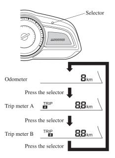
When the ignition is switched to ACC or off, the odometer or trip meters cannot be displayed, however, pressing the selector can inadvertently switch the trip meters or reset them during an approximate ten-minute period in the following cases:
