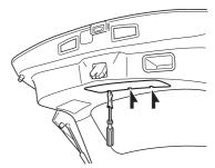
3. Turn the socket and bulb assembly anticlockwise and remove it.
