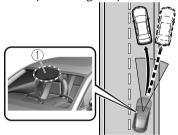
1. Forward sensing camera (FSC)
