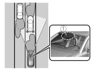
1. Forward Sensing Camera (FSC)\*1
