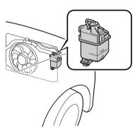
If it is at or near LOW, add enough coolant to the coolant reservoir to provide freezing and corrosion protection and to bring the level to FULL.
