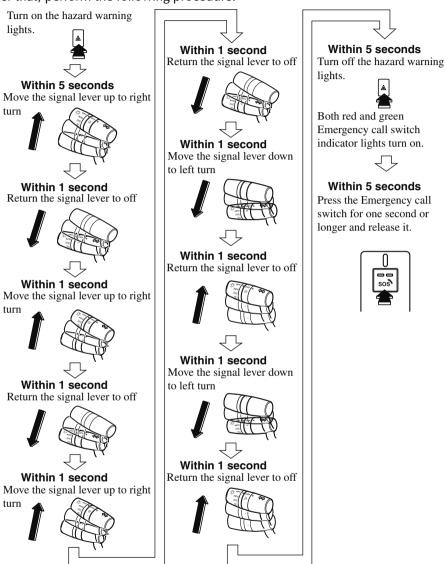
After the procedure is completed, the test mode is performed in the following order automatically.
