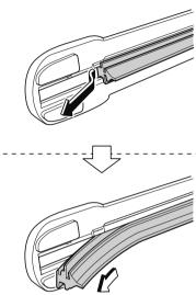
Insert the end of the new blade rubber into the groove of the blade holder until it contacts the end of the blade holder.
