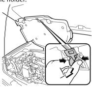
4. Hook the strap onto the bonnet hook to secure the cover.
