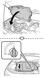
4. Make sure that the engine cover is securely closed.
