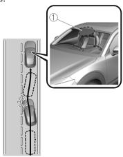
1. Forward sensing camera (FSC)
