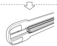
5. Pull the end of the blade rubber from the blade holder groove in the direction of the arrow and remove
