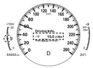
The average fuel economy and trip meters can be reset by pressing the INFO switch for 1.5 seconds or more while in each mode. After the data is cleared, the fuel consumption is recalculated and the - - - L/100 km (- - - mpg) for the 1 minute prior to it being displayed is indicated.
