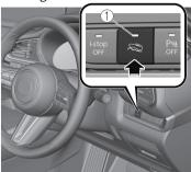
1. Off-Road Traction Assist switch indicator light
