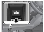
2. Insert your hand into the bonnet opening, slide the latch lever to the left, and lift up the bonnet.
