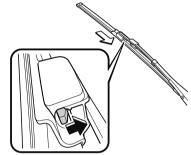
4. Pull the blade rubber in the direction of the arrow and slide it to a position where the blade holder groove can be checked.
