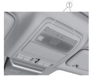
1. Intrusion sensor and intrusion sensor bezel
