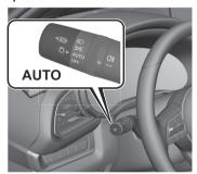
The HBC determines the surrounding conditions and operates automatically. When the HBC operates, the HBC indicator light (green) in the instrument cluster turns on.
