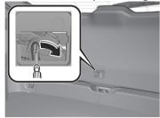
The liftgate is unlocked. After performing this emergency measure, have the vehicle inspected by an expert repairer (we recommend an Authorised Mazda Repairer).
