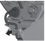
7. Turn the socket and bulb assembly anticlockwise and remove it.
