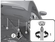
6. Remove the wiring harness from the clip.
