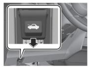
Insert your hand into the bonnet opening, slide the latch lever in the direction of the arrow as shown in the illustration, and lift up the bonnet.
