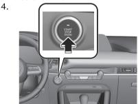
The engine starts and the KEY indicator light (green) " in the instrument cluster turns off.
