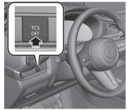
The TCS operation is cancelled and the TCS OFF indicator light of in the instrument cluster and the TCS OFF switch indicator light turn on. Press the TCS OFF switch again to enable the TCS operation.
