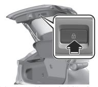
All the doors, liftgate, fuel-filler flap, and the fuel-filler flap are locked. (With theft-deterrent system
