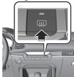
The rear window defogger operates and the switch indicator light turns on. The rear window defogger stops automatically after it operates for about 15 minutes.
