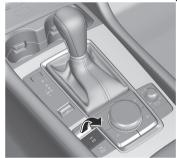
When the shift-linked release is enabled, a sound is activated 2 times, the EPB switch indicator light switches to fast flashing, and then flashes for a certain period of time. When the shift-linked release is disabled, a sound is activated 1
