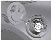
6. Place the fuel-filler cap on the fuel-filler flap holder.
