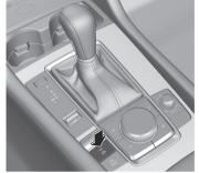
When the parking brake is released, the EPB indicator light (P) in the instrument cluster and the EPB switch indicator light turn off.
