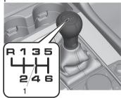
1. Neutral position (**R position**) Operate the shift lever while pushing it down.
