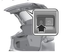
The doors, liftgate, and the fuel-filler flap are locked, the hazard warning lights operate 1 time.
