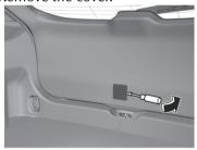
Move the lever. (Vehicles with power liftgate)
