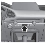
All the direction indicator lights flash and the direction indicator light in the instrument cluster flashes. Press the switch again to turn off the lights.
