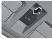
To stop it partway, press the tilt/slide switch.
