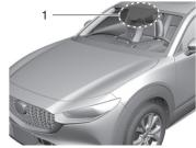
1. Forward Sensing Camera (FSC)
