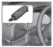
When the ALH is cancelled, the ALH indicator light (green) in the instrument cluster turns off. Press the ALH switch again to make the ALH operable.
