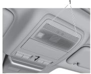
1. Intrusion sensor and intrusion sensor bezel
