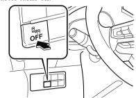
If the switch is pressed again, the BSM and Rear Cross Traffic Alert (RCTA) systems become operable and the BSM OFF indicator light turns off.
