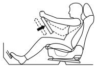
2. Adjust the steering wheel height so that the gauges can be viewed easily.
