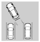
2. After the vehicle starts entering the parking space, stop and adjust the steering wheel so that the distance between the vehicle width lines and the sides of the parking space on the left and right are roughly equal, and then continue backing up slowly.
