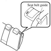
2. Press the seatback rearward and lock it in place. After returning the seatback to its upright position, make sure it is securely locked.
