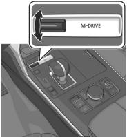
2. While checking the list displayed in the instrument cluster, push the Mi-Drive switch forward or pull it toward you to select a drive mode.
