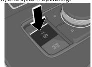
When the parking brake is released, the EPB indicator light (P) in the instrument cluster and the EPB switch indicator light turn off.
