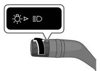
The headlights, position lights, tail lights, and the number plate lights turn on, and the position lights indicator light in the instrument cluster turns on.
