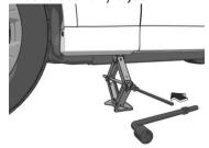
Turn the jack handle clockwise and raise the vehicle high enough so that the spare tyre can be installed. Before removing the wheel nuts, make sure your Mazda is firmly in position and that it cannot slip or move.
