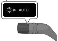
The daytime running lights turn on automatically when it is bright, and the headlights, position lights, tail lights, and the number plate lights turn on automatically when it is dark. When the position lights, tail lights, and the number plate lights are turned on, the position lights indicator light in the instrument cluster turns on.
