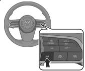
When the system is on, the ISA standby indication (white) LIM is displayed on the screen.
