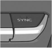
The mode switches between independent mode and interconnection mode each time the switch is pressed.
