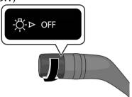
The position lights, tail lights, and number plate lights turn on, and the position lights indicator light in the instrument cluster turns on.
