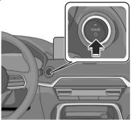
The hybrid system stops and the vehicle power is switched OFF.
