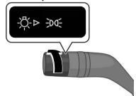
The position lights, tail lights, and number plate lights turn on, and the position lights indicator light in the instrument cluster turns on. When the vehicle power is switched OFF while the position lights, tail lights, and the number plate lights are turned on, the position lights, tail lights, and the number plate lights turn off.
