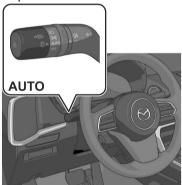
The HBC determines the surrounding conditions and operates automatically. When the HBC operates, the HBC indicator light (green) in the instrument cluster turns on.
