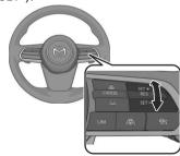
When you set the speed, the set speed is displayed on the screen. In addition, the ISA standby indication (white) LIM changes to the ISA set indication (green) LIM.
