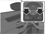
Press the adjustment switch to adjust the angle of the outside mirror.
