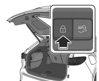
The doors, liftgate, and the fuel-filler flap/charging port lid are locked, the hazard warning lights operate 1 time. Then, the liftgate fully closes automatically.
