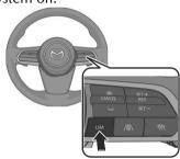
When the system is on, the ASL standby indication (white) LIM is displayed on the screen.
