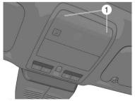
1. Intrusion sensor and intrusion sensor bezel
