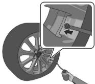
10.Hold the bottom of the bottle upright, squeeze the bottle with your hands, and inject the entire amount of tyre sealant into the tyre.
