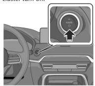
The hybrid system starts and the KEY indicator light (green) [1] in the instrument cluster turns off.
