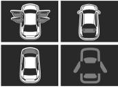
The light turns on if any door/liftgate/bonnet is not closed securely.
