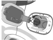
8. Place the fuel-filler cap on the fuel-filler flap holder.
