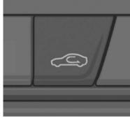
The mode is switched between recirculate mode and fresh air mode each time the switch is pressed. The display indicates whether recirculate mode (<a>) or fresh air mode (<a>) is selected.
