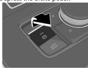
The parking brake is applied and the EPB indicator light (P) in the instrument cluster and the EPB switch indicator light turn on.
