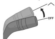
The windscreen wipers operate while the lever is in the position.
