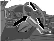
3. Pull up the lever to securely lock the steering wheel.
