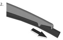
3. Remove the metal stiffeners from the blade rubber and install them in the new blade rubber.
