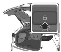
All the doors, liftgate, fuel-filler flap, and the fuel-filler flap/charging port lid are locked.
