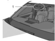
1. Forward Sensing Camera (FSC)
