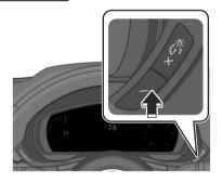
If you press the - switch again while the instrument panel illumination is at maximum dimness, a sound is activated to notify you that the dimmer setting is at maximum dimness.
