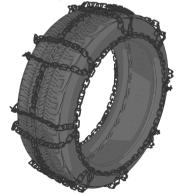
Although Mazda recommends hexagon type steel ring chains, all chains within the installation specifications may be used.
