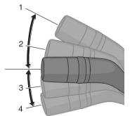
While the lever is in the 2 or 3 position, each direction indicator light flashes and the direction indicator light in the instrument cluster flashes. If you move the lever to the 2 or 3 position and release it immediately, the three-flash turn signal operates and
