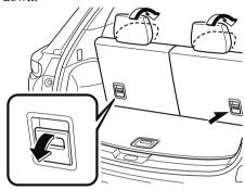
To return the head restraint to its upright position, lift it upward.
