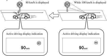
The excessive speed warning is initially set to inoperable. If you want to activate the excessive speed warning, change the setting in the personalisation features. In addition, the warning pattern and the warning activation timing differ depending on the setting contents. Refer to the Settings section in the Mazda Connect Owner's Manual.
