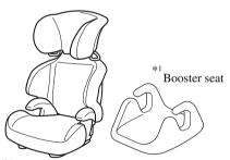
\*1 When using a booster seat, always install the vehicle head restraint to the seat where the booster seat is installed.
