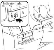
When the ignition is switched ON, the system goes on standby.
