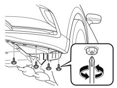
4. Pull the centre of each plastic retainer and remove the retainers, and then partially peel back the mudguard.
