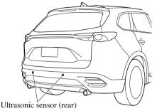
The ultrasonic sensors (rear) are mounted in the rear bumper.
