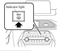
Do not use sharp instruments or window cleaners with abrasives to clean the inside of the rear window surface. They may damage the defogger grid inside the window.
