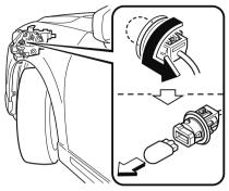
8. Install the new bulb in the reverse order of the removal procedure.
