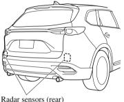
The radar sensors (rear) are installed inside the rear bumper, one each on the left and right sides.
