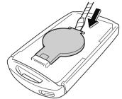
6. Remove the battery using tape-wrapped flathead screwdriver.
