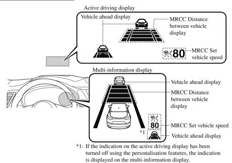
If there is a problem with the MRCC with Stop & Go function system, a message is displayed on the multi-information display. Check the centre display to verify the problem and then have your vehicle inspected by an expert repairer (we recommend an Authorised Mazda Repairer).
