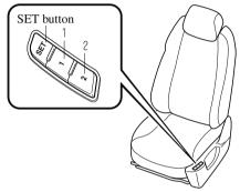
A driving position can be programmed or operated using the buttons on the side of the seat or the key.
