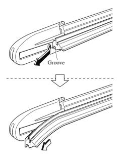
5. Insert the end of the new blade rubber into the groove of the blade holder until it contacts the end of the blade holder.
