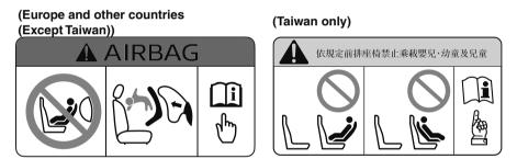
Even in a moderate collision, the child-restraint system can be hit by a deploying air bag and moved violently backward resulting in serious injury or death to the child.
