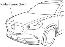
If "Front radar blocked" is displayed in the multi-information display of the instrument cluster, clean the area around the radar sensor (front).
