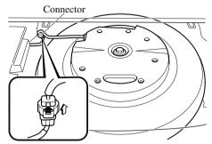
(Vehicles with sub-woofer) Turn the hold-down bolt anticlockwise and remove the sub-woofer and the spare tyre.
