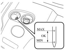
5. Pull it out again and examine the level. The level is normal if it is between the MIN and MAX marks.
