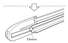
4. Pull the end of the blade rubber from the blade holder groove in the direction of the arrow and remove the blade rubber from the blade holder.
