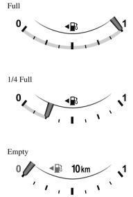
If the fuel level is low, (**•**) and (**0**) turn an amber colour. Refuel as soon as possible. If inconsistency in engine performance or stalling occurs due to low fuel level conditions, refuel the vehicle as soon as possible and add at least 10 L (2.7 US gal, 2.2 Imp gal) of fuel.
