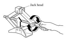
Set the jack to the designated jack-up position closest to the tyre being removed.
