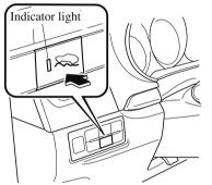
If the switch is pressed again, the Off-Road Traction Assist is stopped and the Off-Road Traction Assist indicator light and the Off-Road Traction Assist switch indicator light turn off.
