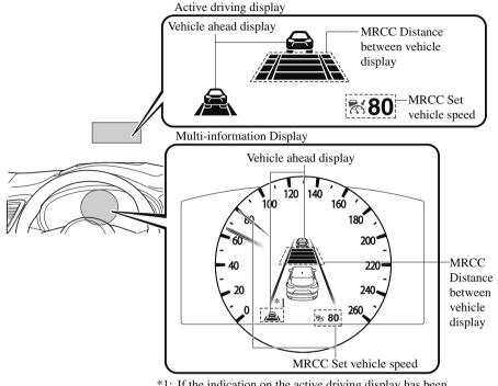
\*1: If the indication on the active driving display has been turned off using the personalisation features, the indication is displayed on the multi-information display.
