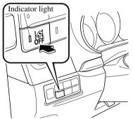
Drive the vehicle in the centre of the driving lane while the LAS & LDWS OFF switch indicator light is turned off.
