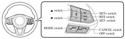
When the MODE switch is pressed once, the MRCC system turns on, and the MRCC main indication (white) turns on and the vehicle speed and the distance between the vehicles while in headway control can be set.
