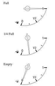
If the low fuel warning light illuminates or the fuel level is very low, refuel as soon as possible. If inconsistency in engine performance or stalling occurs due to low fuel level conditions, refuel the vehicle as soon as possible and add at least 10 L (2.7 US gal, 2.2 Imp gal) of fuel.
