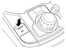
If the EPB switch is pressed without depressing the brake pedal, the display in the instrument cluster notifies the driver that the brake is not depressed.
