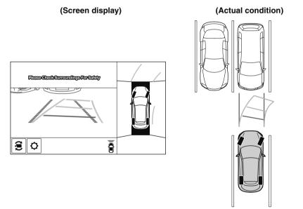
Make sure that there are no obstructions within the projected vehicle path lines. Drive the vehicle forward while turning the steering wheel so that no obstructions come within the projected vehicle path lines.
