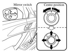
After adjusting the mirror, lock the control by rotating the switch to the centre position.
