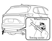
4. Hook the towing rope to the towing eyelet.
