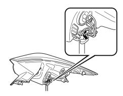
6. Turn the socket and bulb assembly anticlockwise and remove it.
