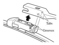
9. Align the blade component projection with the wiper arm notch.
