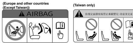
(Taiwan, except front passenger seat, if equipped with the following label) The highly-visible labels warn against the use of a rear-facing child-restraint system on the seat protected by an air bag.
