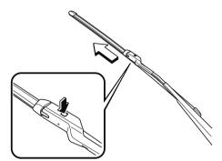
3. Pull the blade rubber in the direction of the arrow and slide it to a position where the blade holder groove can be checked.
