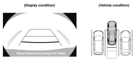
6. When the selector lever is shifted from reverse (R) position to another selector lever position, the screen returns to the previous display.
