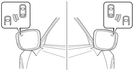
When the ignition is switched ON, the warning indicator light turns on momentarily and then turns off after a few seconds.
