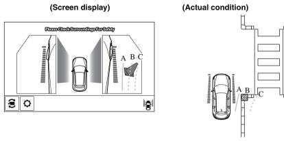
Make sure that there are no obstructions within the projected vehicle path lines. Turn the steering wheel so that the projected vehicle path lines travel inside of the obstruction (A), and drive the vehicle forward until it passes the obstruction. If the projected vehicle path lines are on an obstruction (B) or outside of the obstruction (C), the vehicle may contact the obstruction when turning the vehicle sharply.
