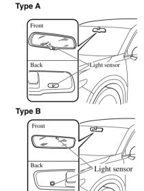
The auto-dimming function is cancelled when the ignition is switched ON and the selector lever is in reverse (R).
