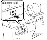
Press the switch again to turn the TCS back on. The TCS OFF indicator light and TCS OFF switch indicator light will turn off.
