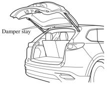
Do not modify or replace the liftgate damper stay. Consult an expert repairer (we recommend an Authorised Mazda Repairer) if a liftgate damper stay is deformed or damaged for reasons such as a collision or if there is some other problem.
