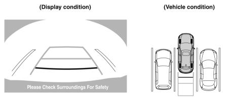
6. When the selector lever is shifted from reverse (R) position to another selector lever position, the screen returns to the previous display.
