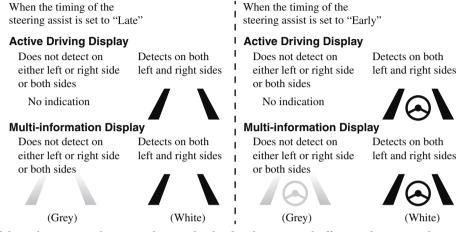
If the indication on the active driving display has been turned off using the personalisation features, the LAS & LDWS indication on the multi-information display is displayed in grey and the system goes on standby.
