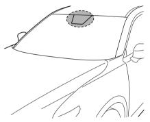
The Forward Sensing Camera (FSC) determines the conditions ahead of the vehicle while travelling at night and detects traffic lanes. The distance in which the Forward Sensing Camera (FSC) can detect objects varies depending on the surrounding conditions.
