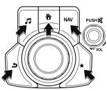
The following operations can be done by pressing the switches around the commander knob.
