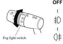
The headlight switch must be in the  $\exists 0 0 \exists 0$  position when turning on the front fog lights.
