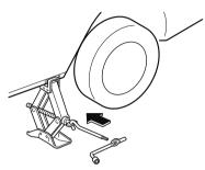
Turn the jack handle clockwise and raise the vehicle high enough so that the spare tyre can be installed. Before removing the wheel nuts, make sure your Mazda is firmly in position and that it cannot slip or move.
