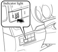
The LAS & LDWS OFF switch indicator light turns on.
