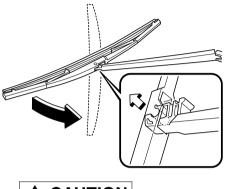
To prevent damage to the rear window, do not let the wiper arm fall on it.
