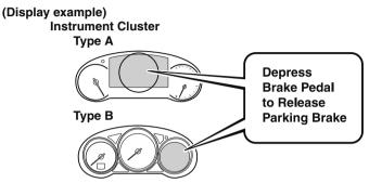
If the warning light turns on/flashes simultaneously or a symbol is indicated in the display, check the information regarding the warning light or symbol.
