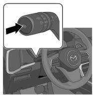
When the ALH is cancelled, the ALH indicator light (green) (in the instrument cluster turns off. Press the ALH switch again to make the ALH operable.
