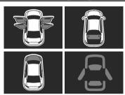
The light turns on if any door/liftgate/bonnet is not closed securely. Close the door/liftgate/bonnet securely.
