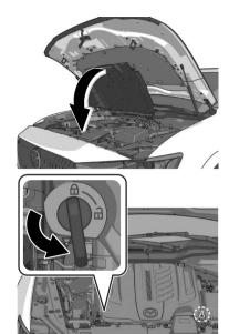
5. Make sure that the engine cover is securely closed.
