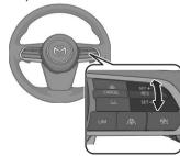
When you set the speed, the set speed is displayed on the screen. In addition, the ISA standby indication (white) Changes to the ISA set indication (green) LIM.
