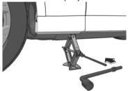
7. Turn the jack handle clockwise and raise the vehicle high enough so that the spare tyre can be installed. Before removing the wheel nuts, make sure your Mazda is firmly in position and that it cannot slip or move.
