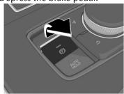
The parking brake is applied and the EPB indicator light (P) in the instrument cluster and the EPB switch indicator light turn on.
