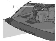
1. Forward Sensing Camera (FSC)
