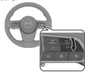
When you set the speed, the set speed is displayed on the screen. In addition, the ASL standby indication (white) Changes to the ASL set indication (green) LIM.
