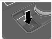
The AUTOHOLD becomes operational and the AUTOHOLD standby indicator light turns on.
