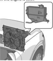
If it is at or near the LOW position, add enough coolant to the coolant reservoir to provide freezing and corrosion protection and to bring the level to FULL.
