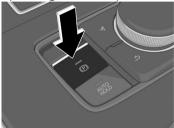
After the parking brake auto operation is cancelled, a warning sound is activated one time, and the EPB switch indicator light switches from illumination to flashing, and then turns off after a certain period of time has passed.
