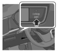
The i-stop function stops and the i-stop OFF switch indicator light turns on.
