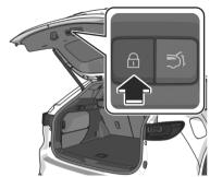
The doors, liftgate, and the fuel-filler flap are locked, the hazard warning lights operate 1 time.
