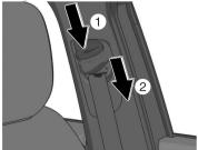
2. Make sure that the seat belt anchor adjuster is securely locked.
