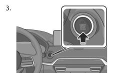
The engine stops and the vehicle power is switched OFF.
