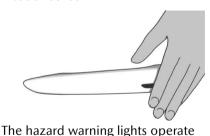
once, and all the doors, liftgate, fuel-filler flap are locked. (Except European models)
