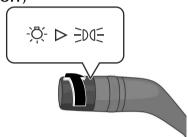
The position lights, tail lights, side-marker lights, and number plate lights turn on, and the position lights indicator light in the instrument cluster turns on.
