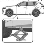
5. Continue raising the jack head gradually by rotating the screw with your hand until the jack head is inserted into the jack-up position.
