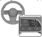
Constant speed driving starts when the vehicle speed is set. In addition, the set speed is displayed on the screen, and the CTS standby indication (white) changes to the CTS set indication (green).
