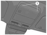
Intrusion sensor and intrusion sensor bezel
