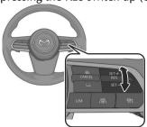
Constant speed driving starts when the vehicle speed is set. In addition, the set speed is displayed on the screen, and the MRCC standby indication (white) changes to the MRCC set indication (green).
