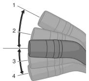
While the lever is in the 2 or 3 position, each direction indicator light flashes and the direction indicator light in the instrument cluster flashes. If you move the lever to the 2 or 3 position and release it immediately, the three-flash turn signal operates and the direction indicator light flashes 3 times
