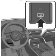
The rear window defogger operates and the switch indicator light turns on. The rear window defogger stops automatically after it operates about 15 minutes.
