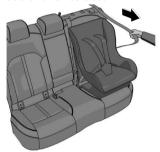
7. Push the child-restraint system firmly into the vehicle seat. Be sure the belt retracts as snugly as possible. A clicking noise from the retractor will be heard during retraction if the system is in the automatic locking mode. If the belt does not lock the seat down tight, repeat this step.
