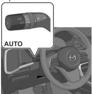
The HBC determines the surrounding conditions and operates automatically. When the HBC operates, the HBC indicator light (green) hin the instrument cluster turns on.
