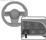
When the system is on, the ASL standby indication (white) LIM is displayed on the screen.
