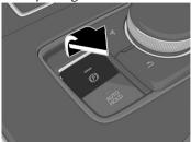
The brakes are applied and the vehicle can be decelerated/stopped. A sound is activated when the brake is applied and when the EPB switch is released, the brake will be released and the sound stops.
