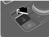
When the shift-linked release is enabled, a sound is activated 2 times, the EPB switch indicator light switches to fast flashing, and then flashes for a certain period of time. When the shift-linked release is disabled, a sound is activated 1 time, the EPB switch indicator light switches to slow flashing, and then flashes for a certain period of time.
