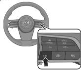
When the system is on, the ISA standby indication (white) IM is displayed on the screen.
