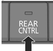
The indicator light turns on and the screen changes to the rear
