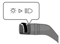
The headlights, position lights, tail lights, side-marker lights, and the number plate lights turn on, and the position lights indicator light in the instrument cluster turns on.
