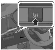
The TCS operation is cancelled and the TCS OFF indicator light of in the instrument cluster and the TCS OFF switch indicator light turn on. Press the TCS OFF switch again to enable the TCS operation.
