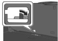
The liftgate is unlocked. After performing this emergency measure, have the vehicle inspected by an expert repairer (we recommend an Authorised Mazda Repairer).
