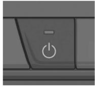
Switches the air-conditioning system on and off.
