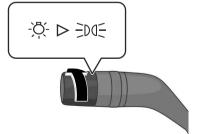
The position lights, tail lights, side-marker lights, and number plate lights turn on, and the position lights indicator light in the instrument cluster turns on.
