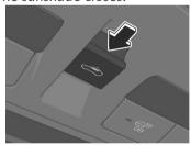
To stop it partway, operate the switch in the direction opposite to the direction it is opening/closing.
