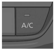
The cooling/dehumidifying function switches between on and off each time the switch is pressed. The indicator light turns on while the function is operating.
