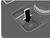
The AUTOHOLD operation is cancelled and the AUTOHOLD standby indicator light turns off.
