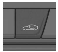
The mode is switched between recirculate mode and fresh air mode each time the switch is pressed.
