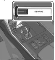
2. While checking the list displayed in the instrument cluster, push the Mi-Drive switch forward or pull it toward you to select a drive mode. Instrument cluster (Type A)
