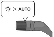
The daytime running lights turn on automatically when it is bright, and the headlights, position lights, tail lights, side-marker lights\*, and the number plate lights turn on automatically when it is dark.
