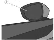
Objects visible outer and inner sections of the wide-angle mirror are at different distances. Objects that displayed in the outer section are actually farther away than the inner section.
