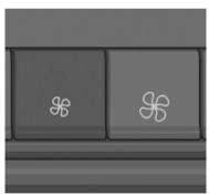
The airflow amount changes each time the switch is pressed. The airflow amount is indicated on the display. The airflow amount can be adjusted to 7 levels.
