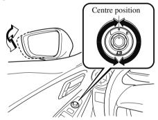
**Type B**To fold the mirrors, press the ₱ mark on the outside mirror folding switch.
