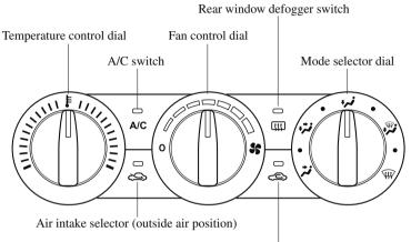
Air intake selector (recirculated air position)
