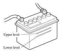
Inspect the electrolyte level at least once a week. If it is low, remove the caps and add enough distilled water to bring the level between the upper and lower level (illustration).
