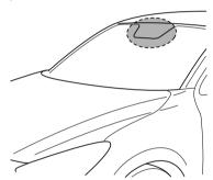
The Forward Sensing Camera (FSC) determines the conditions ahead of the vehicle while travelling at night and detects traffic lanes. The distance in which the Forward Sensing Camera (FSC) can detect objects varies depending on the surrounding conditions.
