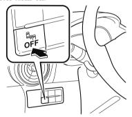
If the switch is pressed again, the BSM and Rear Cross Traffic Alert (RCTA) systems become operable and the BSM OFF indicator light turns off.
