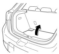
2. Turn the spare tyre hold-down bolt anticlockwise.
