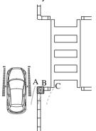
Make sure that there are no obstructions within the projected vehicle path lines. Turn the steering wheel so that the projected vehicle path lines travel inside of the obstruction (A), and drive the vehicle forward until it passes the obstruction. If the projected vehicle path lines are on an obstruction (B) or outside of the obstruction (C), the vehicle may contact the obstruction when turning the vehicle sharply.
