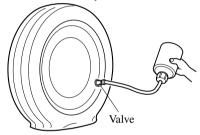
11. Pull out the injection hose from the valve.
