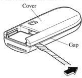
Twist the flathead screwdriver in the direction of the arrow and remove the cover
