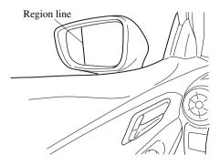
• The perceived distance of objects in the outer and inner regions of the wide angle mirror is different. Objects appearing in the outer region are actually further away than they are in the inner region.
