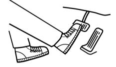
Wear shoes appropriate for driving in order to avoid your shoe contacting the brake pedal when depressing the accelerator pedal.
