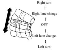
The direction indicators in the instrument cluster flash according to the operation of the direction indicator lever to show which
