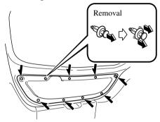
3. Using a flathead screwdriver, open the inner cover.
