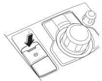
Firmly depress the brake pedal and press the electric parking brake switch. If the electric parking brake switch is pressed without depressing the brake pedal, the indicator light in the instrument cluster notifies the driver that the brake is not depressed.
