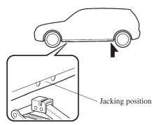
Continue raising the jack head gradually by rotating the screw with your hand until the jack head is inserted into the jack-up position.
