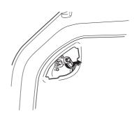
4. Disconnect the connector from the unit by pressing the tab on the connector with your finger and pulling the connector.
