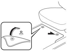
When setting a floor mat, position the floor mat so that its grommets or retainers are inserted over the pointed end of the retention posts.
