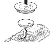
6. Insert a new battery with the positive pole facing up, and then cover the battery with the battery cap.
