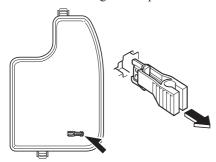
4. Inspect the fuse and replace it if it is blown.
