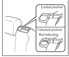
1. Make sure that the seat belt passes through the seat belt guide correctly and it is not twisted, then raise the seatback while preventing the seat belt from being caught in the seatback. (Saloon)
