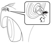
4. Turn the socket and bulb assembly to remove it. Carefully remove the bulb from its socket in the reflector by gently pulling it straight backward out of the socket.
