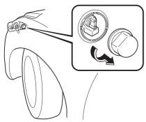
4. Turn the socket and bulb assembly anticlockwise and remove it.
