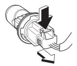
5. Disconnect the bulb by pulling it out. Rear direction indicator lights, Brake lights/Tail lights (Bulb type)
