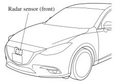
If "SBS, MRCC, DRSS Radar blocked" is displayed in the multi-information display of the instrument cluster, clean the area around the radar sensor (front).
