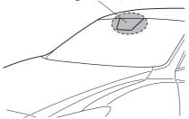
The Forward Sensing Camera (FSC) determines the conditions ahead of the vehicle while travelling at night and detects traffic lanes. The distance in which the Forward Sensing Camera (FSC) can detect objects varies depending on the surrounding conditions.
