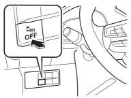
If the switch is pressed again, the Blind Spot Monitoring (BSM) and Rear Cross Traffic Alert (RCTA) systems become operable and the Blind Spot Monitoring (BSM) OFF indicator light turns off.
