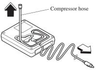
8. Install the compressor hose which was pulled out of the air compressor to the injection valve of the bottle.
