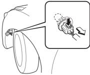
6. Turn the socket and bulb assembly anticlockwise and remove it.
