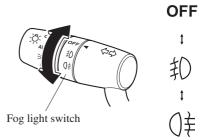
The headlight switch must be in the ₹00€ or ≣○ position when turning on the front fog lights.
