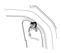
Disconnect the connector from the unit by pressing the tab on the connector with your finger and pulling the connector.
