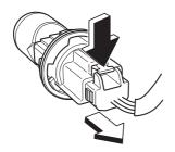
7. Disconnect the bulb by pulling it out. Rear direction indicator lights, Brake lights/Tail lights/Rear side-marker lights (Bulb type)
