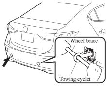
4. Hook the towing rope to the towing eyelet.
