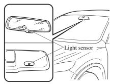
The auto-dimming function is cancelled when the ignition is switched ON and the shift/selector lever is in reverse (R).
