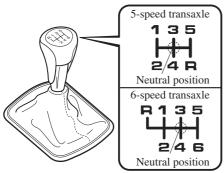
The vehicle is equipped with either a 5-speed or 6-speed transaxle. The shift pattern for each is shown above.
