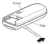
Twist the flathead screwdriver in the direction of the arrow and remove the cover.
