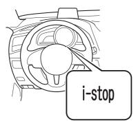
• The i-stop indicator light (green) turns off when the engine is restarted.
