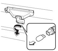
7. Install the new bulb in the reverse order of the removal procedure.
