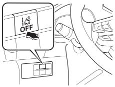
The Lane-keep Assist System (LAS) & Lane Departure Warning System (LDWS) OFF indicator light turns on.
