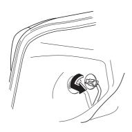
7. Disconnect the connector from the unit by pressing the tab on the connector with your finger and pulling the connector.
