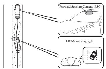
The warning light flashes when the system has a malfunction. Refer to Warning Lights on page 4-42.
