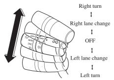
The direction indicators in the instrument cluster flash according to the operation of the direction indicator lever to show which signal is working.
