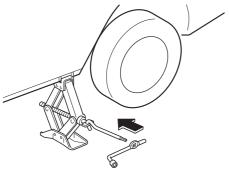
8. Turn the jack handle clockwise and raise the vehicle high enough so that the spare tyre can be installed. Before removing the wheel nuts, make sure your Mazda is firmly in position and that it cannot slip or move.
