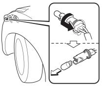
8. Install the new bulb in the reverse order of the removal procedure.
