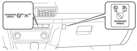
The front passenger air bag deactivation switch should be used to deactivate the front passenger front and side air bags and also the front passenger seat belt pretensioner system if installing a child-restraint system on the front passenger seat.
