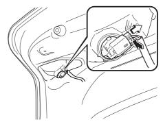
5. Turn the socket and bulb assembly anticlockwise and remove it.
