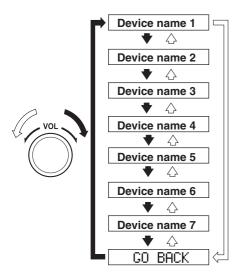
Press the audio control dial to select the device you would like to link.
