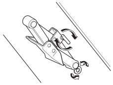
11. Turn the wing bolt completely to secure the jack.
