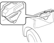
If it is at or near L, add enough coolant to the coolant reservoir to provide freezing and corrosion protection and to bring the level to F.
