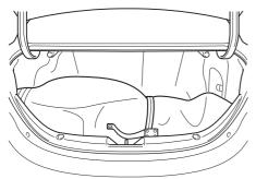
2. Place the second golf bag in the boot with its bottom pointed to the left and fit it into the back of the boot.
