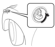
5. Install the new bulb in the reverse order of the removal procedure.
