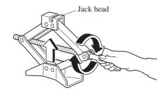
5. Place the jack under the jack-up position closest to the tyre being changed with the jack head squarely under the jack-up point.
