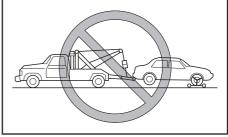
If towing service is not available in an emergency, the vehicle may be towed with all four wheels on the ground using the towing hook at the front of the vehicle. Only tow the vehicle on paved surfaces for short distances at low speeds.
