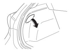
Turn the socket and bulb assembly anticlockwise and remove it.
