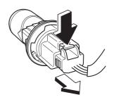
8. Disconnect the bulb by pulling it out. Rear direction indicator lights, Brake lights/Tail lights/Rear side-marker lights (Bulb type)
