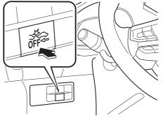
Press the switch again to turn the system back on. The Smart City Brake Support (SCBS) OFF indicator light will turn off.
