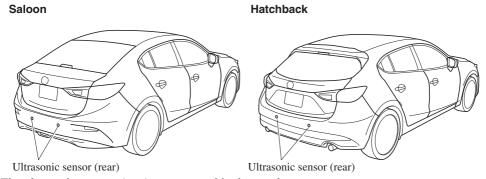
The ultrasonic sensors (rear) are mounted in the rear bumper.
