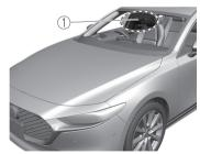
1. Forward Sensing Camera (FSC)
