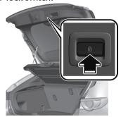
When locking using the door-lock switch, press the door-lock switch with all of the following conditions met and then close the liftgate.
