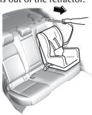
5. Push the child-restraint system firmly into the vehicle seat. Be sure the belt retracts as snugly as possible. A clicking noise from the retractor will be heard during retraction if the system is in the automatic locking mode. If the belt does not lock the seat down tight, repeat this step.
