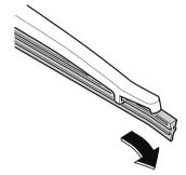
3. Remove the metal stiffeners from the blade rubber and install them in the new blade.
