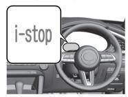
The i-stop indicator light (green) turns off when the engine is restarted.
