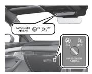
The front passenger air bag deactivation switch should be used to deactivate the front passenger front and side air bags and also the front passenger seat belt pretensioner system if installing a child-restraint system on the front passenger seat.
