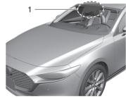
1. Forward Sensing Camera (FSC)
