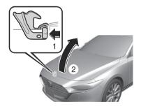
3. Grasp the support rod in the padded area and secure it in the support rod hole indicated by the arrow to hold the bonnet open.
