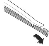
3. Remove the metal stiffeners from the blade rubber and install them in the new blade rubber.
