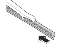
5. Install the blade assembly in the reverse order of removal.
