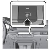
The rear window defogger operates and the switch indicator light turns on. The rear window defogger stops automatically after it operates for about 15 minutes.
