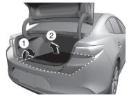
2. Turn the spare tyre hold-down bolt anticlockwise and remove the spare tyre.
