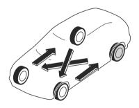
Do not include (TEMPORARY USE ONLY) spare tyre in rotation. Also, inspect them for uneven wear and damage. Abnormal wear is usually caused by one or a combination of the following:
