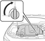
5. Make sure that the engine cover is securely closed.
