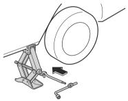
Turn the jack handle clockwise and raise the vehicle high enough so that the spare tyre can be installed. Before removing the wheel nuts, make sure your Mazda is firmly in position and that it cannot slip or move.
