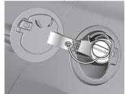
6. Place the fuel-filler cap on the fuel-filler flap holder.
