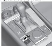
The parking brake is applied and the EPB indicator light (P) in the instrument cluster and the EPB switch indicator light turn on.
