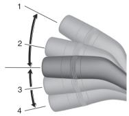
Each direction indicator light flashes and the direction indicator light in the instrument cluster flashes. The lever returns to its original position in conjunction with the steering wheel operation. If it does not return, return it by hand.
