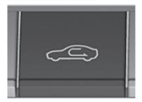
The mode is switched between recirculate mode and fresh air mode each time the switch is pressed. The display indicates whether recirculate mode (((a)) or fresh air mode ((a)) is selected.
