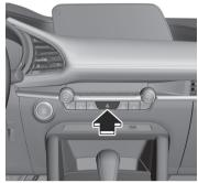
All the direction indicator lights flash and the direction indicator light in the instrument cluster flashes. Press the switch again to turn off the lights.
