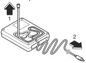
14.Install the compressor hose to the tyre valve.
