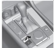
When the shift-linked release is enabled, a sound is activated 2 times, the EPB switch indicator light switches to fast flashing, and then flashes for a certain period of time. When the shift-linked release is disabled, a sound is activated 1
