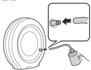
10.Hold the bottom of the bottle upright, squeeze the bottle with
