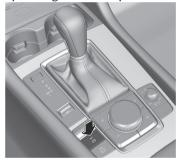
After the parking brake auto operation is cancelled, a warning sound is activated one time, and the EPB switch indicator light switches from illumination to flashing, and then turns off after a certain period of time has passed.
