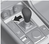
2. Pull the up switch (+/OFF) or the down switch (-) of the steering shift switches toward you.
