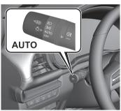
The ALH operates automatically after determining the surrounding conditions.
