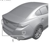
1. Rear side radar sensors (Hatchback) Vehicle front
