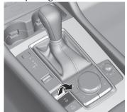
The brakes are applied and the vehicle can be decelerated/stopped. A sound is activated when the brake is applied and when the EPB switch is released, the brake will be released and the sound stops.
