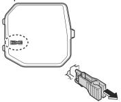
4. Inspect the fuse and replace it if it is blown.
