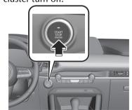
The engine starts and the KEY indicator light (green) " in the instrument cluster turns off.
