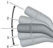
While the lever is in the 2 or 3 position, each direction indicator light flashes and the direction indicator light
