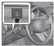
The TCS/DSC operation is cancelled and the DSC OFF indicator light in the instrument cluster and the DSC OFF switch indicator light turn on. Press the DSC OFF switch again to enable the TCS/DSC operation.
