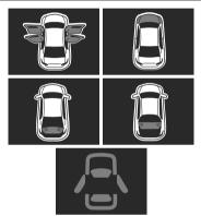
The light turns on if any door/boot lid/liftgate/bonnet is not closed securely.
