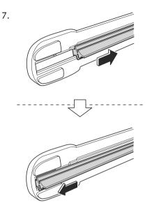
8. Make sure that the blade rubber is correctly installed to the blade holder. 9.
