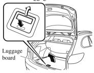
2. Turn the spare tyre hold-down bolt anticlockwise.
