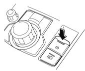
If the EPB switch is pressed without depressing the brake pedal, the display in the instrument cluster notifies the driver that the brake is not depressed. A message is displayed on the multi-information display in the instrument cluster.
