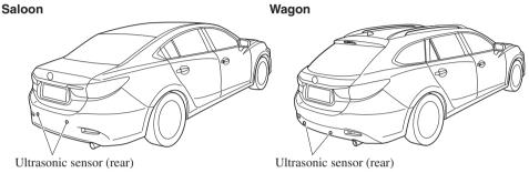
The ultrasonic sensors (rear) are mounted in the rear bumper.
