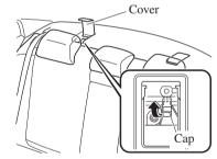
3. **(European models)** Turn the screw anticlockwise and remove it, and then remove the theft-prevention cover.
