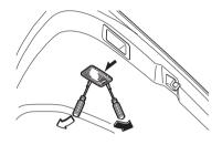
2. Disconnect the electrical connector from the bulb by pressing the tab on the connector with your finger and pulling the connector.
