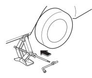
7. Turn the jack handle clockwise and raise the vehicle high enough so that the spare tyre can be installed. Before removing the wheel nuts, make sure your Mazda is firmly in position and that it cannot slip or move.
