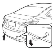
Do not use excessive force as it may damage the cap or scratch the painted bumper surface.
