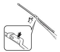
3. Pull the blade rubber in the direction of the arrow and slide it to a position where the blade holder groove can be checked.
