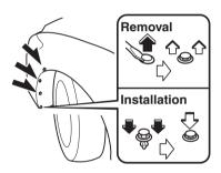
4. Turn the screw anticlockwise and remove it, and then partially peel back the mudguard.
