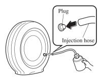
10. Hold the bottom of the bottle upright, squeeze the bottle with your hands, and inject the entire amount of tyre sealant into the tyre.
