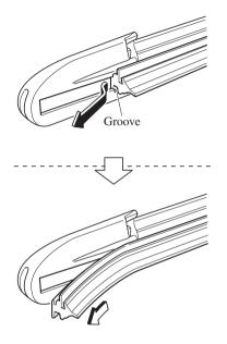
5. Insert the end of the new blade rubber into the groove of the blade holder until it contacts the end of the blade holder.
