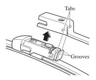
9. Align the blade component projection with the wiper arm notch.
