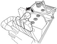
4. Turn off the booster vehicle's engine and connect the jumper leads in the following order.
