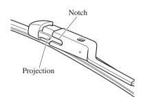
10. Slide the blade component and install it to the wiper arm.
