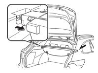
Removing the luggage compartment cover at a slight angle will make it easier to remove.
