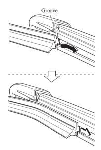
6. After pulling the blade rubber in the direction of the arrow and sliding the blade rubber to a position to check the blade holder groove, slide the blade rubber end in the opposite direction.
