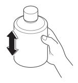
If the bottle is shaken after the injection hose is screwed on, tyre sealant could spray out from the injection hose. Tyre sealant contacting clothing or other objects may be impossible to remove. Shake the bottle before screwing on the injection hose.
