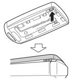
3. Insert a tape-wrapped flathead screwdriver into the gap and slide it in the direction of the arrow.
