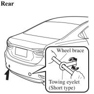
4. Hook the towing rope to the towing eyelet.
