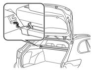
2. Retract the spring holder on the right end of the retractor bar to insert it into the installation groove.
