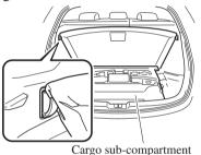
3. Remove the pocket by pulling the tab.
