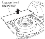
3. Turn the spare tyre hold-down bolt anticlockwise.
