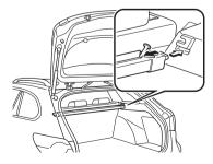
3. Slowly pull out the net in the upward direction, insert the left and right net anchors into the ceiling retainers, and slide them to the position indicated in the figure.
