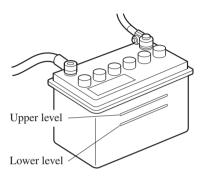
Inspect the electrolyte level at least once a week. If it is low, contact an expert repairer (we recommend an Authorised Mazda Repairer) for the electrolyte level.
