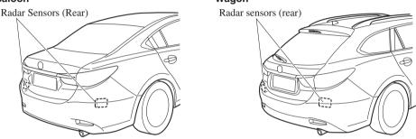
The radar sensors (rear) are installed inside the rear bumper, one each on the left and right sides.
