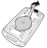
6. Remove the battery using tape-wrapped flathead screwdriver.
