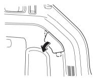
3. Turn the socket and bulb assembly anticlockwise and remove it.
