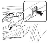
3. If any fuse but the MAIN fuse is blown, replace it with a new one of the same amperage rating.
