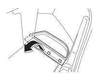
4. Turn the wing bolt and jack screw anticlockwise.
