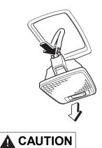
When replacing the bulb always disconnect the connector first. Otherwise, electric and electronic devices could be shorted. 3. Insert the flathead screwdriver into the gap between the lens and the lens unit, and then slide the screwdriver to detach the lens.
