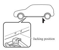
5. Continue raising the jack head gradually by rotating the screw with your hand until the jack head is inserted into the jack-up position.
